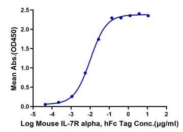
Immobilized Human IL-7, No Tag at 2µg/ml (100µl/well) on the plate. Dose response curve for Mouse IL-7R alpha, hFc Tag with the EC50 of 10.2ng/ml determined by ELISA.
