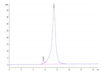
The purity of Mouse IL-7R alpha is greater than 95% as determined by SEC-HPLC.
